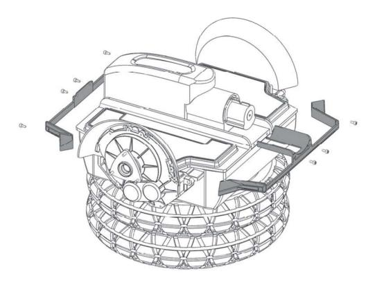
**Step 5:** Carefully stack the wheels and place the Segway® base unit on top of the wheels as a platform to work from. Remove the bumper frames by removing the eight (8) – 4mm Hex screws with the 4mm Hex wrench (included).
