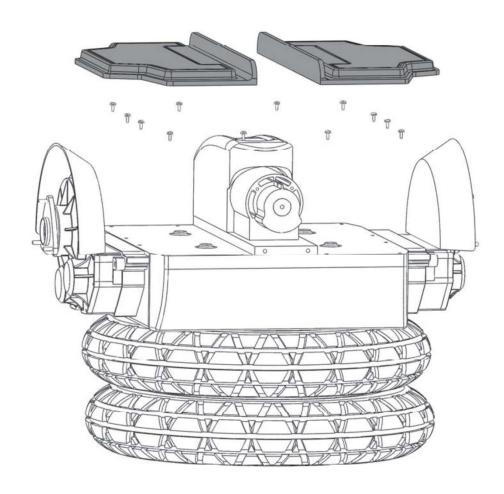
**Step 6:** Remove the floor mats and the twelve (12) plate deck bolts (these bolts will no longer be needed for the ALLY installation) with the T27 wrench (included).
