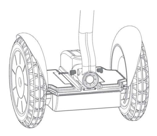
**Step 2:** Remove the locking wedges to disassemble the steer frame by removing the 5mm Hex bolt using the 5mm hex wrench (included with the Segway). (This is already unattached if you have purchased a new Segway®). Keep the locking wedges and bolt.
