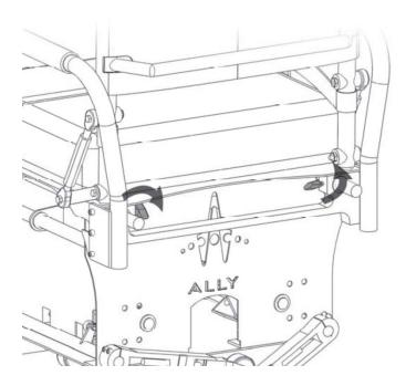
**Step 7:** Loosen the seat plate adjustment knob by turning it counter clock-wise. The knob is located in the middle of the seat pan behind the seat.
