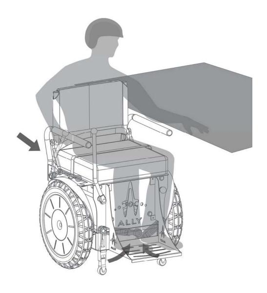
4. Place one hand on a solid surface and in one swift motion, fully retract the Stabilizers by pressing down on the Stabilizer Lever. CAUTION: Slow or partial retraction of the Stabilizers can leave the ALLY unbalanced and lead to falls and injury.
