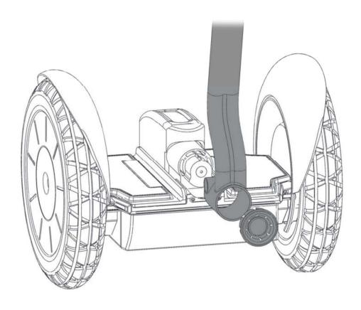
**Step 3:** Remove the Lean Steer Frame. (This is already unattached if you have purchased a new Segway®. The new Segway® may not have the center console cover attached. Attach the center console cover.).
