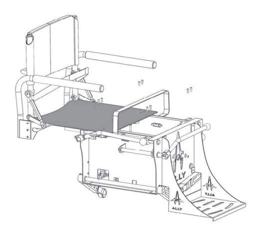
**Step 9:** Remove the eight (8) seat pan bolts with the 4mm wrench (included). Slide off the seat assembly to expose the internals.
