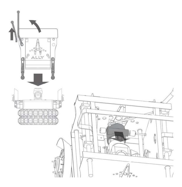
**Step 10:** Ensure the steering lever is vertical and the stabilizer lever is in the deployed position as indicated and mate the ALLY with the Segway®. Slide on the steering hub as indicated.
