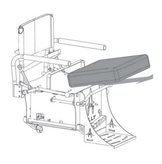
**Step 8:** Remove the seat cushion to expose the seat pan bolts.
