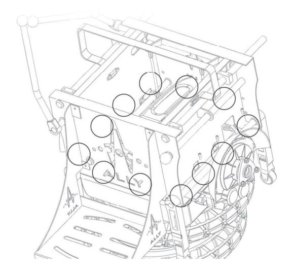
**Step 12:** Fasten the ALLY unit to the Segway® base by installing the twelve (12) 5mm deck bolts (included). First, tighten the deck bolts by hand, and then tighten with the 5mm Hex wrench (included).
