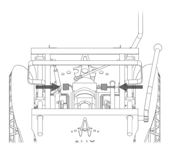
**Step 11:** Ensure the steering lever is vertical and that the steering hub is level prior to the installation of the wedges. Install the locking wedges by tightening the 5mm Hex bolt with the 5mm Hex wrench (included) or by tightening the set screw on top of the steering hub.
