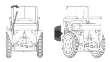
9. Press the steering lever to the left. The ALLY will turn in place to the left. Approximately 7 pounds (3.2 kg) of pressure left and right is required to steer the ALLY.
