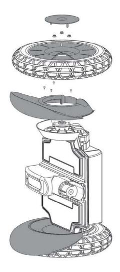
**Step 4:** Flip the Segway® on its side. Remove the Segway® tires and fenders. First, remove the hub with a screw driver or similar (it just pops off). Second, remove the tire by removing the three (3) – 13mm nuts (13mm wrench not included). Third, remove the fender by removing the four (4) - Torx T20 bolts with the T20 wrench (included).
