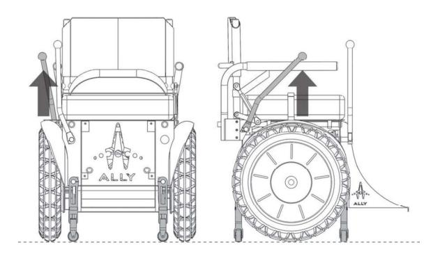
1.1. Place the assembled ALLY on a level surface and deploy the Stabilizers (while not mounted). Do this by lifting UP the Stabilizer Lever until it locks into position.
